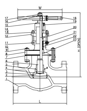
Davis cast steel valves comply with the following applicable specifications: ANSI B16.10, ANSI B16.5, API 600: Tested to API 598
