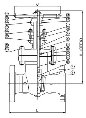
Davis cast steel valves comply with the following applicable specifications: ANSI B16.10, ANSI B16.5, API 600: Tested to API 598
