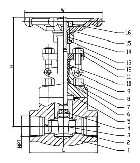
Davis forged steel valves comply with the following applicable specifications: ANSI B16.34, ANSI B16.11, ANSI B1.20.1, API602, API606, MSS SP-84, BS5352: Tested to API 598
