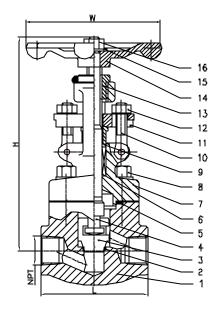
Davis forged steel valves comply with the following applicable specifications: ANSI B16.34, ANSI B16.11, ANSI B1.20.1, API602, API606, MSS SP-84, BS5352: Tested to API 598
