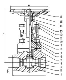
Davis forged stainless valves comply with the following applicable specifications: ANSI B16.34, ANSI B16.11, ANSI B1.20.1, API602, API606, MSS SP-84, BS5352: Tested to API 598
