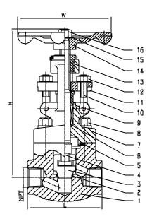
Davis forged stainless valves comply with the following applicable specifications: ANSI B16.34, ANSI B16.11, ANSI B1.20.1, API602, API606, MSS SP-84, BS5352: Tested to API 598
